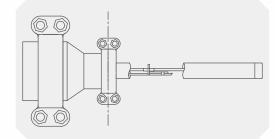
Multipoint thermometer without sheath (installed in sheath)
