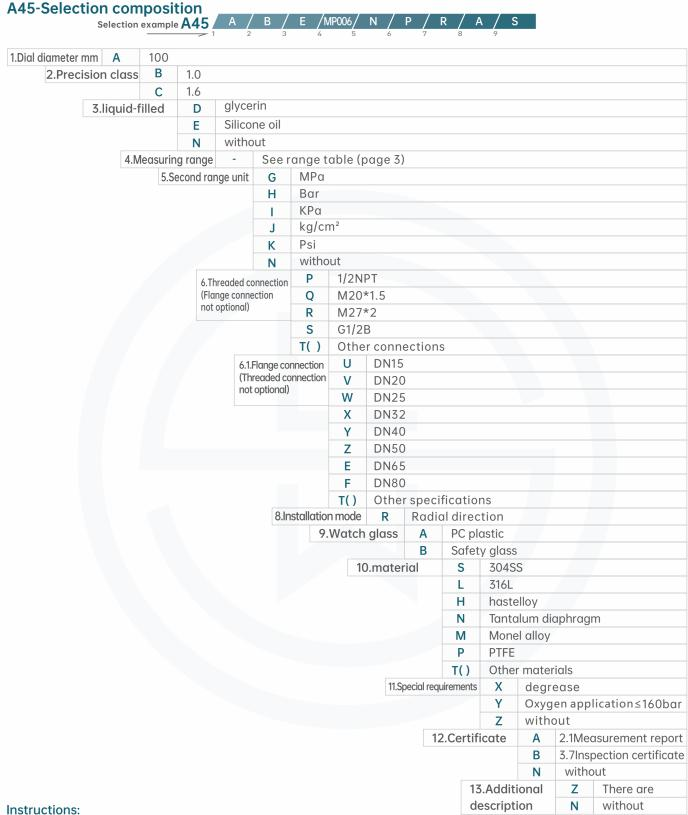
It indicates that A45 pressure gauge dial diameter is 100mm, accuracy level is 1.0%, shockproof filled silicone oil, measuring range is 0~0.6MPa, no second measuring range unit, process connection 1/2NPT(6.6.1 is one of the two options), radial installation, safety glass, body material is 304SS. Item 11/12/13 of the above table is not required.
