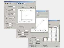
Additional tank volume calculations can be used with DTM functionality to reproduce any optional tank geometry. The corresponding linearized table is automatically generated. Linearized forms can be transferred directly to the transmitter.
