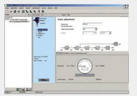
For HART output signals, Profibus-PA and FF, DTM can be used according to the FDT standard. For all transmitter setup and control procedures, DTM provides a self-parsing, clear user interface. When testing, DTM also simulates all process values and archives parameter data. Measurements can be recorded for diagnostic purposes.
