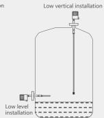
Schematic diagram of ash hopper installation
