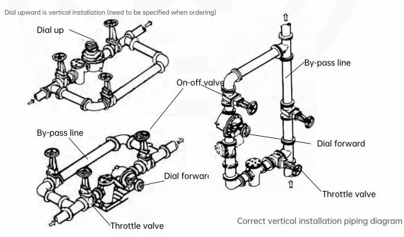
Correct horizontal installation piping diagram
